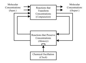
Figure 1: Block diagram of a synchronous sequential system.
