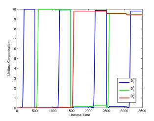
Figure 7: Transient simulation result of the counter.
