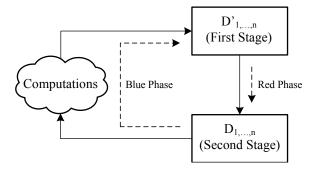
Figure 3: The two-phase memory transfer scheme.
